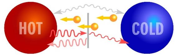
Particle and energy fluxes in junction between hot and cold during electronic cooling.
