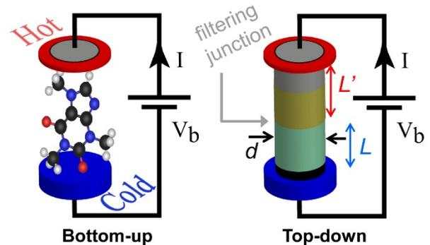
Schematic illustration of the two EFINED approaches in the case of biased detection/ electron cooling. In the bottom-up approach the main engineering tool is synthesis whereas in the top-down approach the selected materials and dimensions  $d$ ,  $L$  and  $L'$  provide similar handle.
